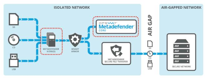
Figure 1: Example TOE deployment
